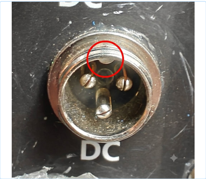
Socket (on the machine and on the battery). The red circle marks the notch in the collar.
